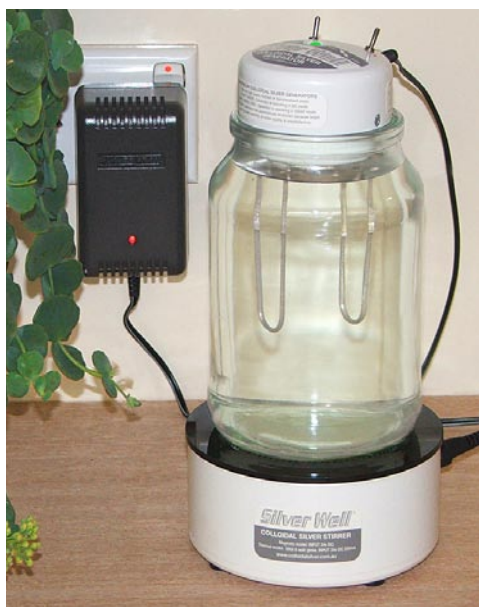
Generator, Stirrer Base, and Transformer.
